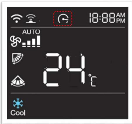
To enable or disable **CONSTANT** function press **CONSTANT** button from the remote. **CONSTANT** Mode can be selected in **COOL**, **DRY**, **FAN** and **HEAT** mode only.
