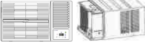
1) Remove the rear screw and save it for later use. Pullout the chassis by grasping the front handle.
