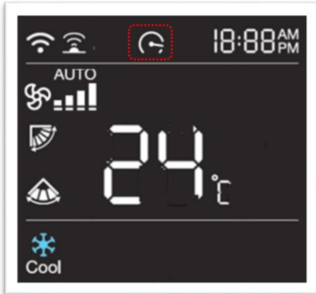
To enable or disable CONSTANT function press CONSTANT button from the remote. CONSTANT Mode can be selected in COOL, DRY and HEAT mode only.
