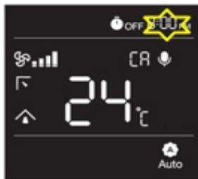
After ON/OFF timer selected and RTC timer will start blinking
