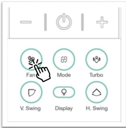
Each time you press the FAN button, FAN SPEED will change as per below cyclic order [\*Depends on the Type of Remote]. Use fan key to increase or decrease the fan speed. Silent fan speed can be selected directly from fan key .
