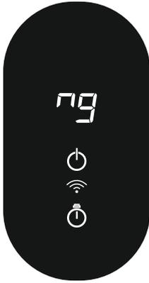
If Emergency / Display button not pressed with in next three-minute, Unit will go back to normal mode.
