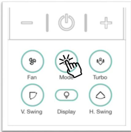
Each time when you press the Mode button, operating mode will change in cyclic order from COOL, DRY, FAN, AUTO & Heat.
