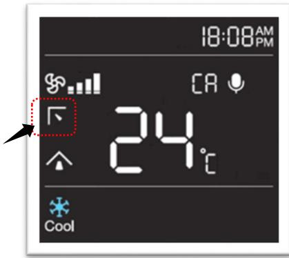
Each time when you press the V SWING button, air flow blade will change as per below cyclic order [\*Depends on the Type of Remote]. The selected swing position will be displayed on the remote handset and the appropriate indication will illuminate on remote handset display.
