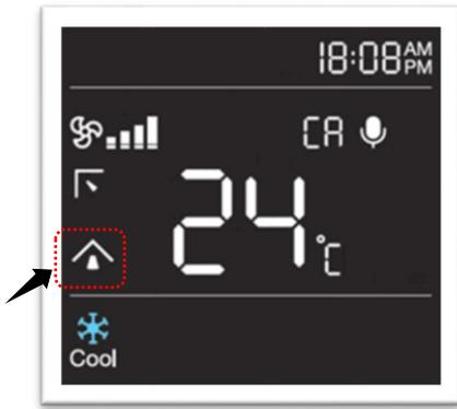
Press H SWING button in the remote handset to enable Auto Swing and icon will appear on remote handset display, press the button again to disable this function and icon will disappear from remote handset display.
