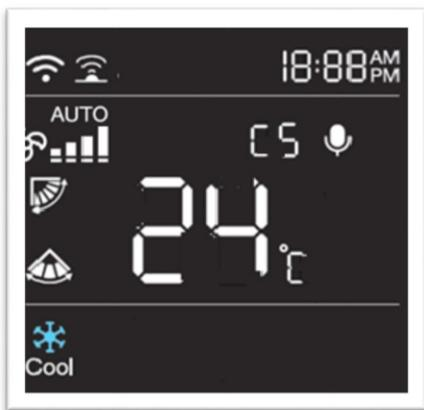
Press 6-in-1 button for the first time, preset selected level will show on remote handset display. Press the button again within 3 seconds to change the capacity as C1, C2, C3, C4, C5 and the respective capacity level will be displayed on the remote handset as well as on indoor display.
